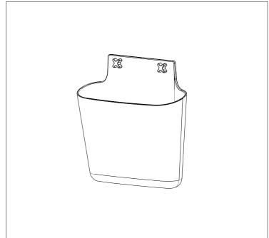
**1** Drill 2 holes on the wall with 6mm dia and 30mm depth. Insert part 4. (Ignore this step if it is wooden wall)
