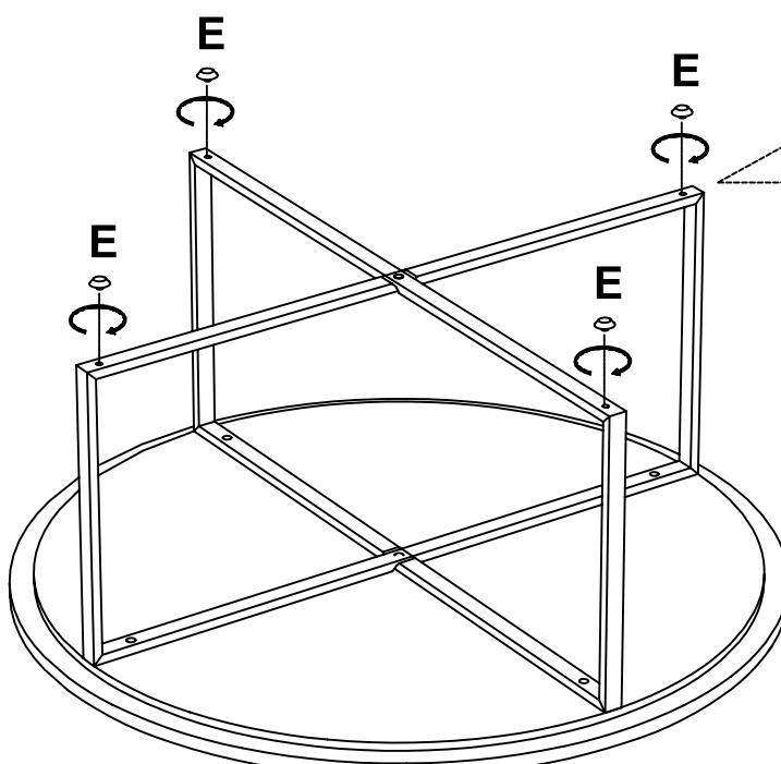
First tighten the four adjustable foot pads , then turn the table upside down . Check that the desktop is flat . If there is any tilt on the table , please adjust the bottom pad corresponding to the tilt direction until the table is flat .
