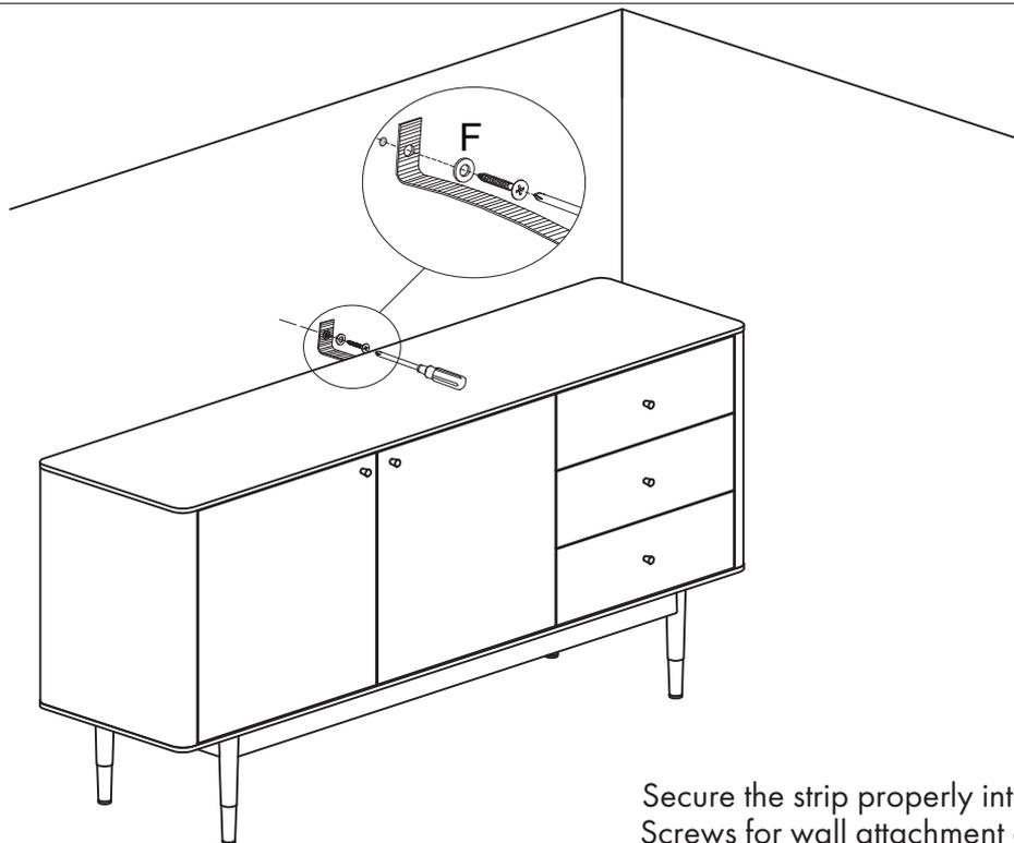
Secure the strip properly into the wall.
