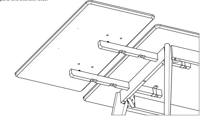
STEP 3: Please tighten the wing screw (using hand) on leaf panel first.
