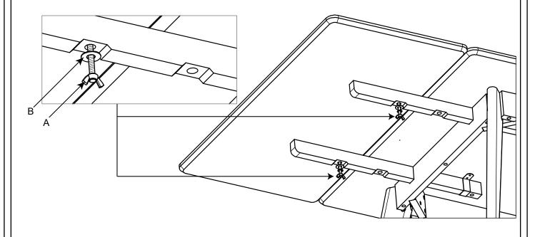
STEP 4: Insert the wing screw on Table side, but before tighten it, push the leaf panel until no gap visible between leaf and top panel, then please ensure all wing screw fully tightened.
