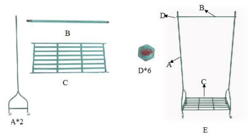
STEP 1: PUT THE PART C BETWEEN AND AT THE BOTTOM OF THE PART A, TIGHTEN IT WITH THE PART D
