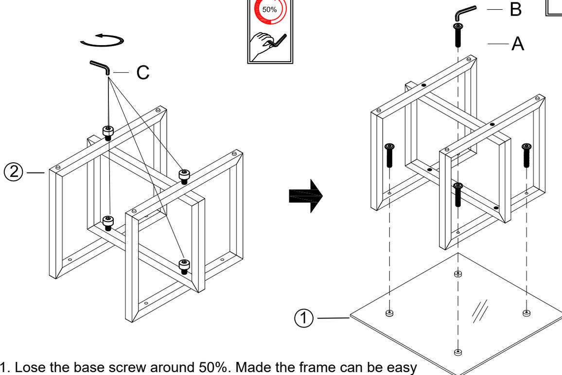
1. Lose the base screw around 50%. Made the frame can be easy to aim at the glass screw hole.
