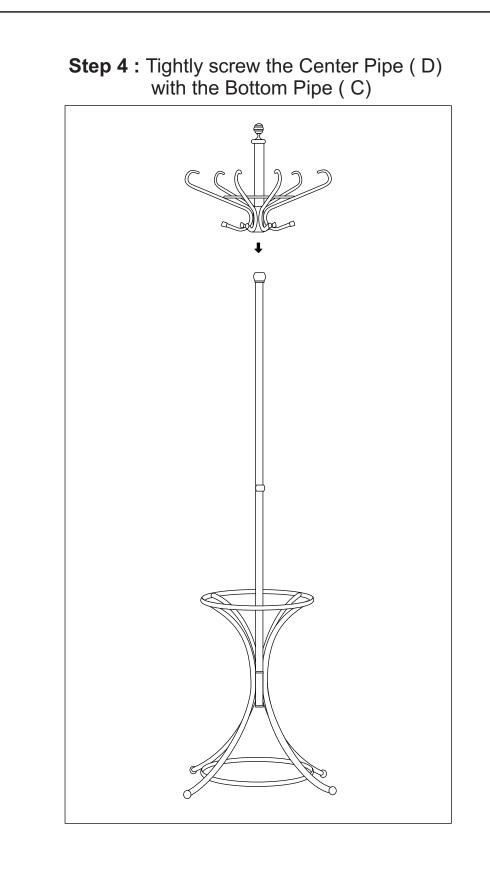
**Note -** At the time of assembly, the hook crown is slid from the top. At the time of assembly, the poles may gather scratches, handle carefully.
