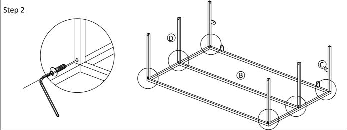
Gently insert the Connector (C) & (D) on to the protruded metal stud on Leg Frame (B) ensuring holes on the connectors aligned with pre-threaded holes on Leg frame (B). Secure connections using 6 Pcs Small Allen Bolt (H3). Do not fully tighten all connections yet.
