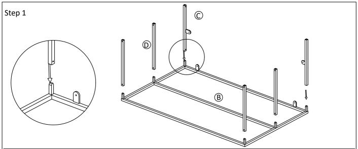
Place Leg Frame (B) on a non-damaging padded surface. Insert Metal Connector (C) on the provided tab of Metal Frame (B) then Insert Metal Connector (D) on the the provided tab of Metal Frame (B) as shown in the picture.
