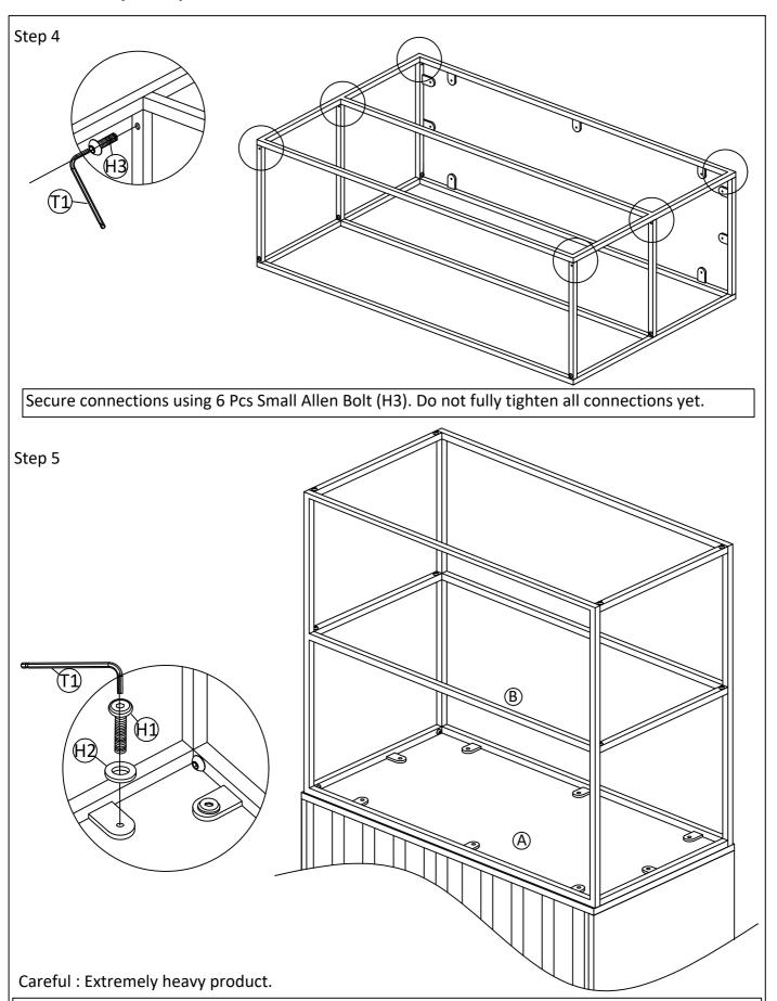
Place Cabinet (A) upside down on a non-damaging padded surface. Place Leg Frame (B) on bottom of Cabinet (A) ensuring holes on the leg frame (B) are aligned with the holes underneath the Desk (A). Secure all connections using 10 Large Allen Bolt (H1) and 10 Washer (H2) on metal tab as shown above. Fully tighten all connections using Allen Key (T1).
