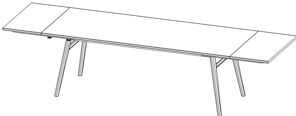
Extension sticks should be fixed to the back of extension plate, when not in use.
