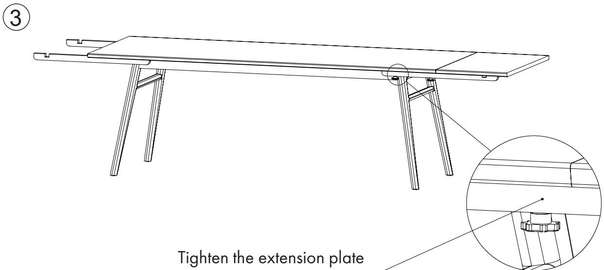
Tighten the extension plate with thumbscrew and get table top and extension in level.
