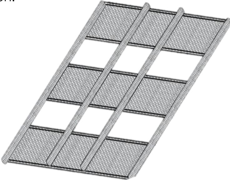
2. Unfold the side panels into the top and bottom shelf.
