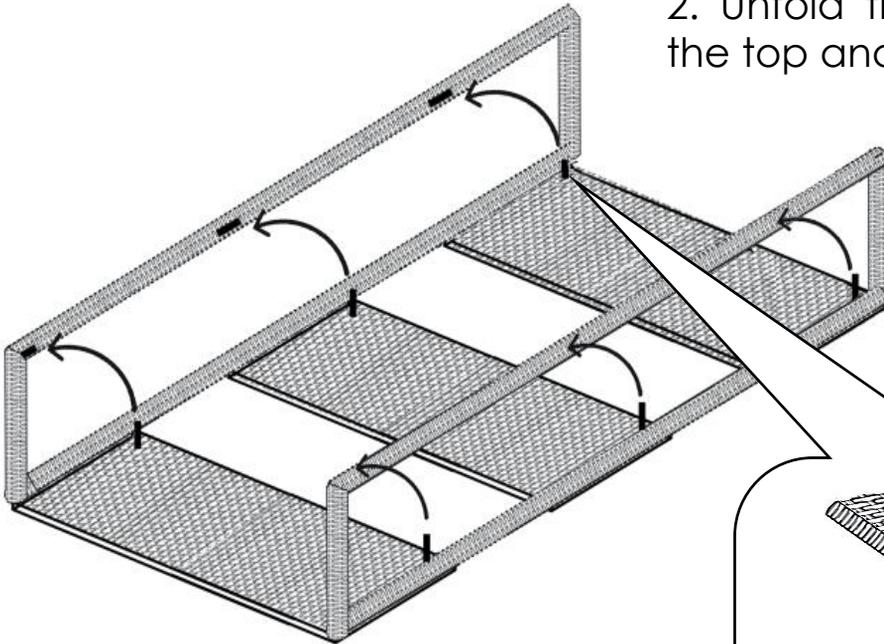
3. Insert top, middle and bottom shelf peg into the holes of the side panels pipe frame as shown.
