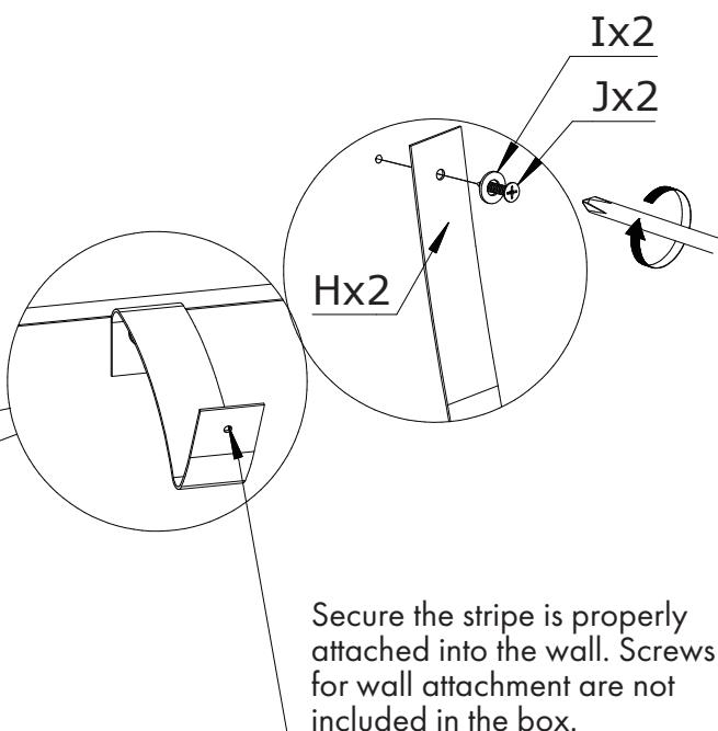
Secure the stripe is properly attached into the wall. Screws for wall attachment are not included in the box.
