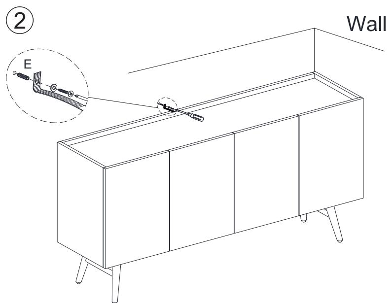
Secure the strip properly into the wall.
