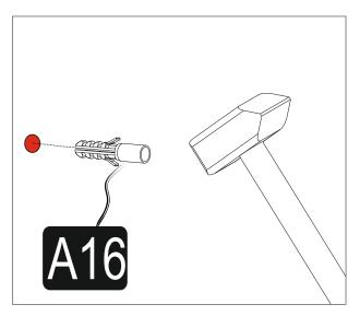
Attach the plugs to the drilled places.
