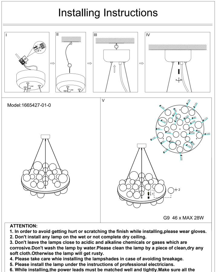
screws are tight enough before turning on the power .Otherwise it will cause the electrical components buring because of the short circuit of the terminals.
