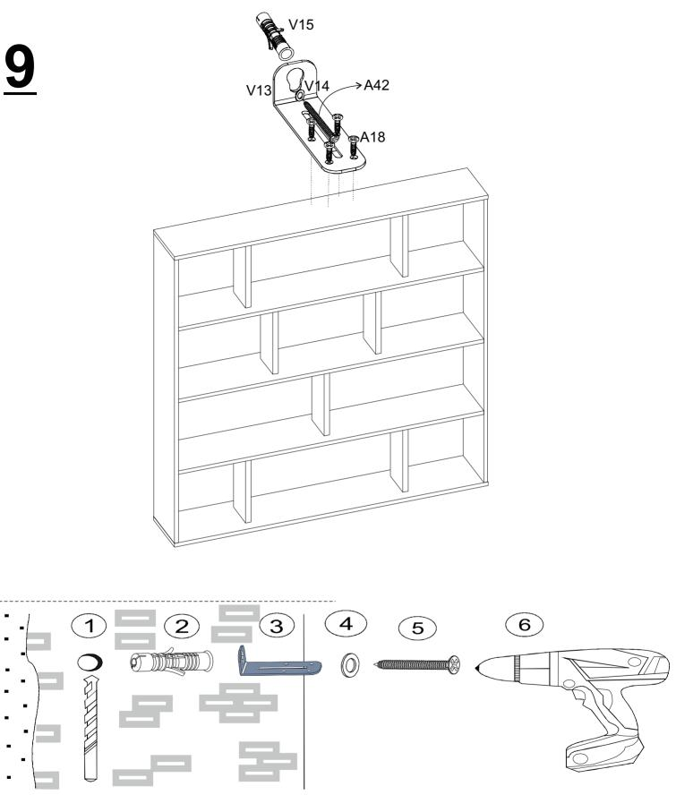
Check the Wall type before installation of dowel. Wall is drilled with equal diameter of dowel.(08mm) Universal Plastic Dowel provides the general purpose usage. Requires two stages assembly. Dowel can be different type according to the wall type. (e.g. Plaster Sheet Partition Wall, Gas Concrete, Hollow Brick Wall) If required, use appropriate dowels and screws.
