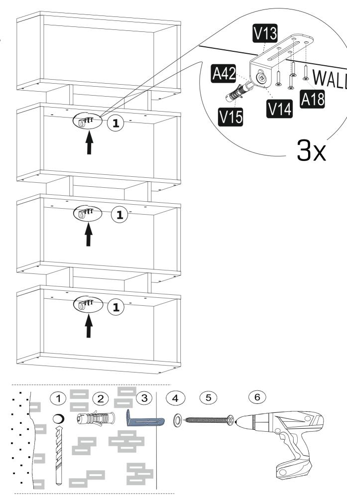
Check the Wall type before installation of dowel. Wall is drilled with equal diameter of dowel.(08mm) Universal Plastic Dowel provides the general purpose usage. Requires two stages assembly.
