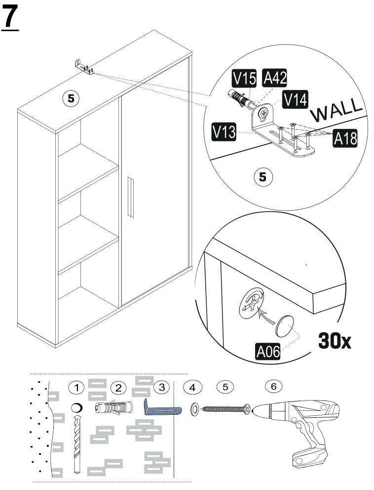
Check the Wall type before installation of dowel. Wall is drilled with equal diameter of dowel.(08mm) Universal Plastic Dowel provides the general purpose usage. Requires two stages assembly. Dowel can be different type according to the wall type. (e.g. Plaster Sheet Partition Wall, Gas Concrete, Hollow Brick Wall) If required, use appropriate dowels and screws.
