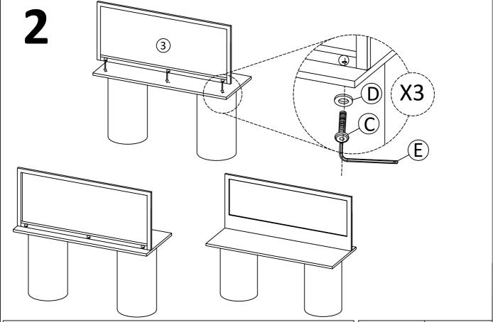
Upright the peace then set the Mirror frame (3) with provided hole on Top (1) as shown in step 3. Ensuring holes on the top (1) are aligned with the holes of Mirror Frame (3). Secure all connections using Allen Bolt (C) Washer (D) as shown above. Fully tighten all connections using Allen Key (E).
