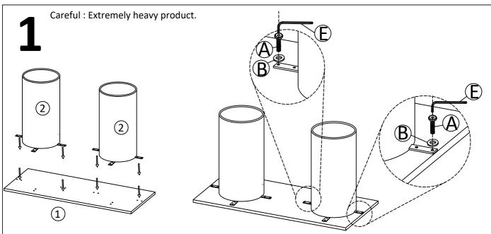
Place Top (1) upside down on a non-damaging padded surface. Place Both round base (2) with metal strip on Top (1) ensuring holes on the top (1) are aligned with the holes of round base (2) as shown in step 1. Secure all connections using Allen Bolt (H1) and Washer (H2) as shown above. Fully tighten all connections using Allen Key (T1) as shown in step 1.
