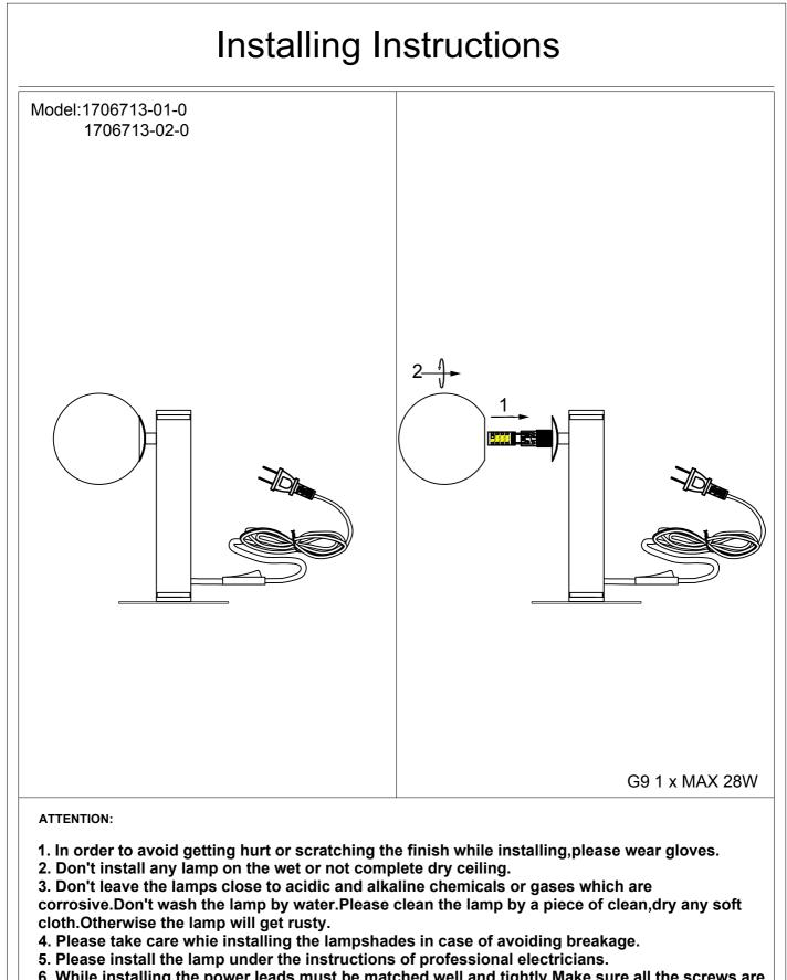
6. While installing, the power leads must be matched well and tightly. Make sure all the screws are tight enough before turning on the power . Otherwise it will cause the electrical components buring because of the short circuit of the terminals.
