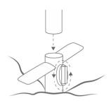
Step 2: Untwist the knob on the sand anchor to allow the center pole of the cabana to be inserted to the anchor.
