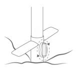
Step 3: Insert middle pole into sand anchor, then twist and turn the knob of the anchor and lock the center pole into place.
