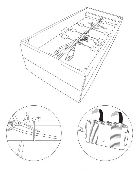
Carefully cut off the plastic straps that hold the wires in place. Detach the transmitter from the holder. Recycle cords, transmitters and remote controls as electrical waste.
