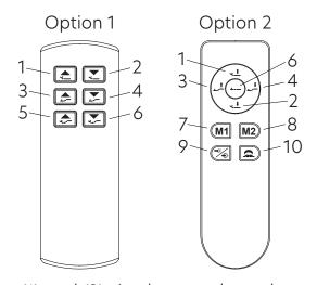
3. Press buttons (1) and (2) simultaneously on the remote control until the LED light starts flashing. When the LED receiver flashes, the connection is complete. Note: The distance between the receiver and the remote control should not be more than two meters during the connection process.
